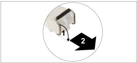
Figure 56: Removing an SFP module
